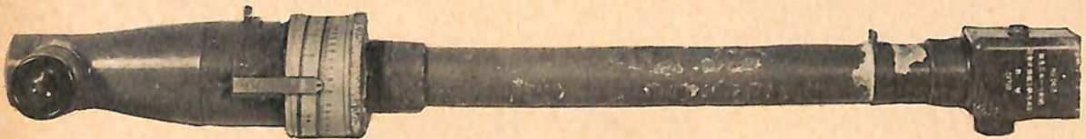
Figure 286. Model 92 (1932) 40-cm base range finder is calibrated for measuring ranges up to 1,500 meters (1,640 yards). It is a coincidence type of range finder with a 4\times magnification.
